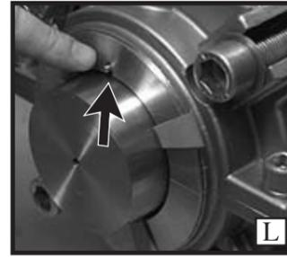
**INSTALLATION INDICATOR / ANTI-ROTATION PIN DETAILS**
